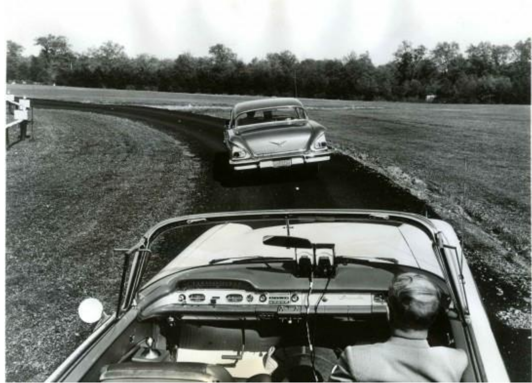
1950s. Autonomous Highway System Tests. GM y RCA developed automated driving prototypes with a radio controller for speed and steering.
